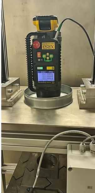
Figure 6. Mobile battery-powered power supply XRS-3 with fixed tungsten anode, with a nominal anode voltage of 270 kV
