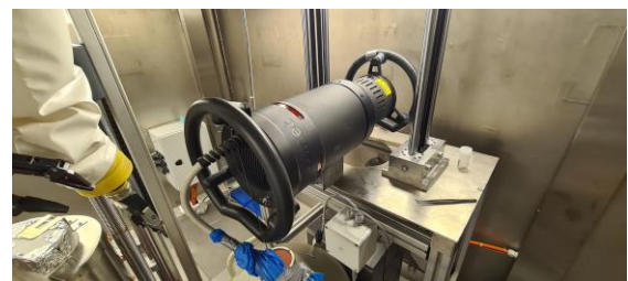
Figure 5. Mobile X-Ray source ECO 200DS with fixed tungsten anode and nominal anode voltage of 200 kV
