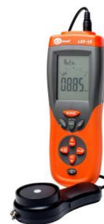
Figure 3. Digital luxmeter Sonel LXP-10A with recording and wireless data transmission
