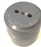
Figure 17. Lead shielding plug with a diameter of 96 mm and a total height of 90 mm, for shielding the mouth of the horizontal channel of the LVR-15 research reactor
