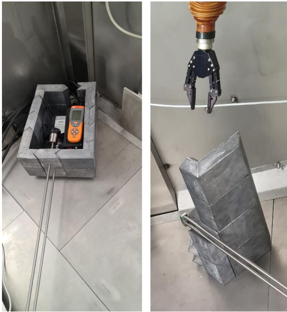
Figure 10. A radiation-shielded lead bunker to protect the probe's sensitive electronics from the effects of ionizing radiation (left), a lead screen to shield the highly active source ^{137}\text{Cs} (right)
