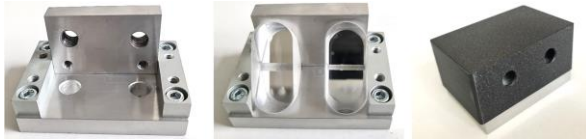
Figure 19. Optical periscope changing the trajectory of the laser beam by 90°
