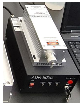
Figure 2. GL532T6-1500 laser source together with ADR-800D control and power supply unit
