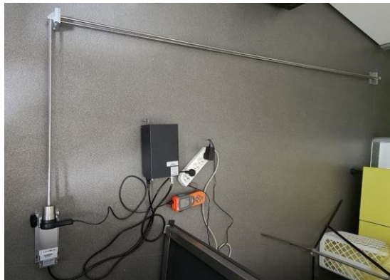
Figure 20. Laboratory testing of the complete laser probe assembly
