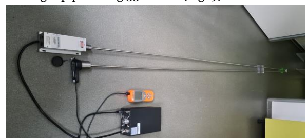
Figure 9. Laboratory tests of assembled probes with a length of light pipes of 3300 mm
