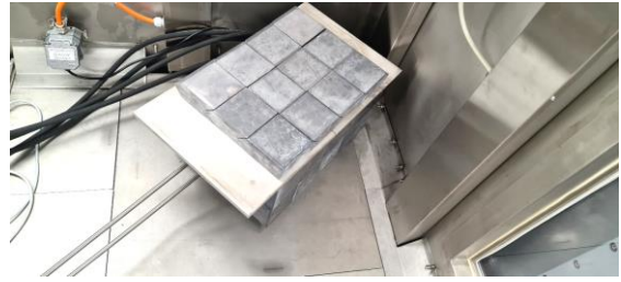
Figure 11. A fully shielded bunker to protect the probe's sensitive electronics from the effects of ionizing radiation
