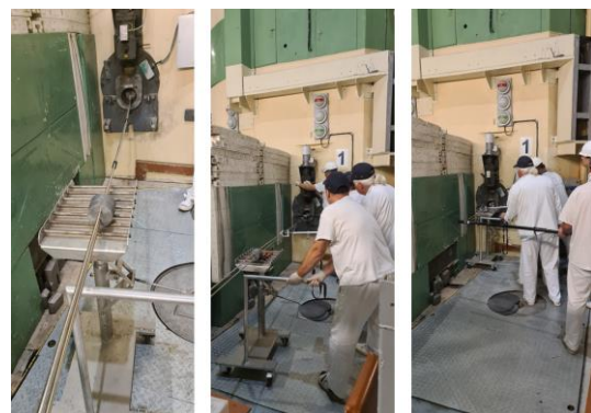
Figure 18. Inserting a 4 m long probe with a lead plug into the horizontal channel of the LVR-15 nuclear research reactor
