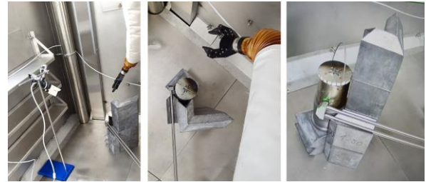
Figure 12. Camera view of the detail of the storage of the high-activity source can behind the shielding screen
