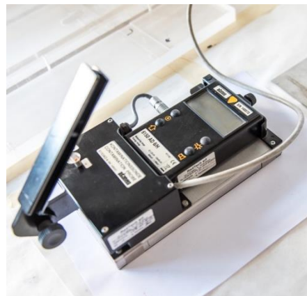
Figure 2. Proportional gas meter used by INMRI for the creation of the national secondary standard of surface emission rate of the WAS.
