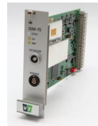
Figure 1. Digital MCA spectrometric module.
