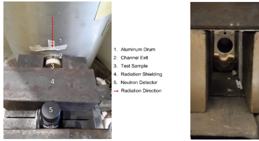
Figure 2. Pu-Be tests setup as seen from above with its main components numbered 1 to 5 (a) and the exit channel seen from the prospective of the neutron detector. The detector's main body is found under the shielding aligned with the exit channel
