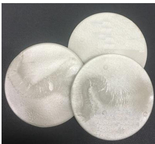
Figure 1. Photograph of doped composite materials produced in the form of a 5 mm thick and 7.5 cm diameter disc
