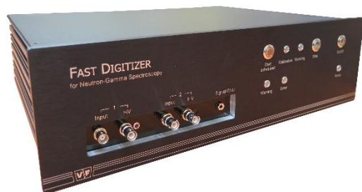
Figure 4. Two-parametric digital neutron-gamma spectrometer NGA-01 [3,4].
