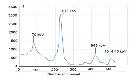
Figure 3. Experimental gamma spectrum of activation detector
