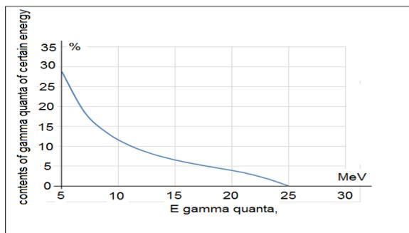
Figure 1. Energy distribution of Bremsstrahlung  $\gamma$ -quanta of Betatron B-25 in Uzhgorod National University
