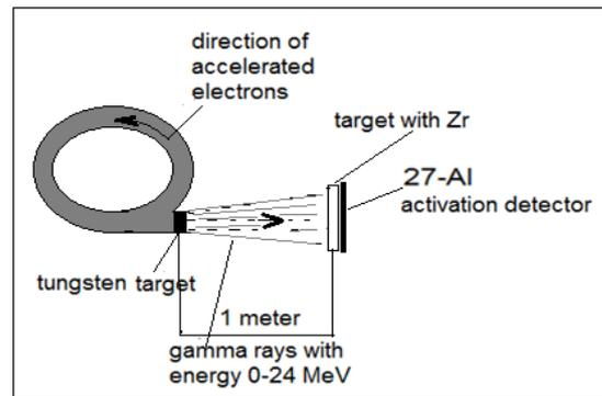
Figure 2. Scheme of targets and activation detector situated
