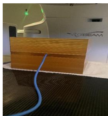
Figure 2. PMMA phantom with TM30013 ionization chamber inserted into a holder
