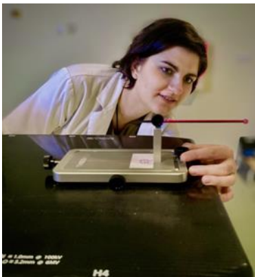
Figure 3. Set-up of ISOBall phantom in accordance with isocenter pointed by laser system
