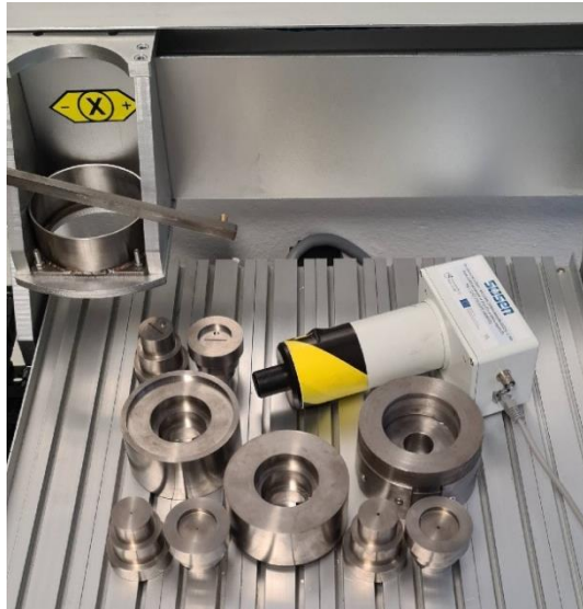
Figure 2. Scintillation detector with collimation system components
