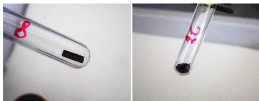
Figure 6. Left – irradiated steel coupon; Right – irradiated titanium scrap
