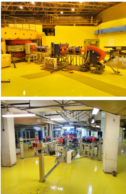
Figure 1. Cyclotron C-80 (ground floor) with three proton beam lines to the target stations (cellar)
